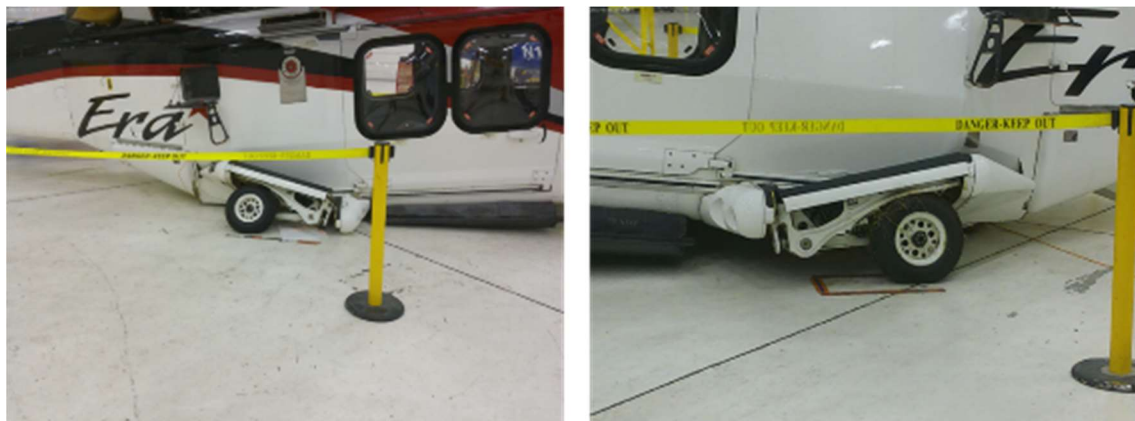
Photo 2: N811TA's collapsed landing gear.
