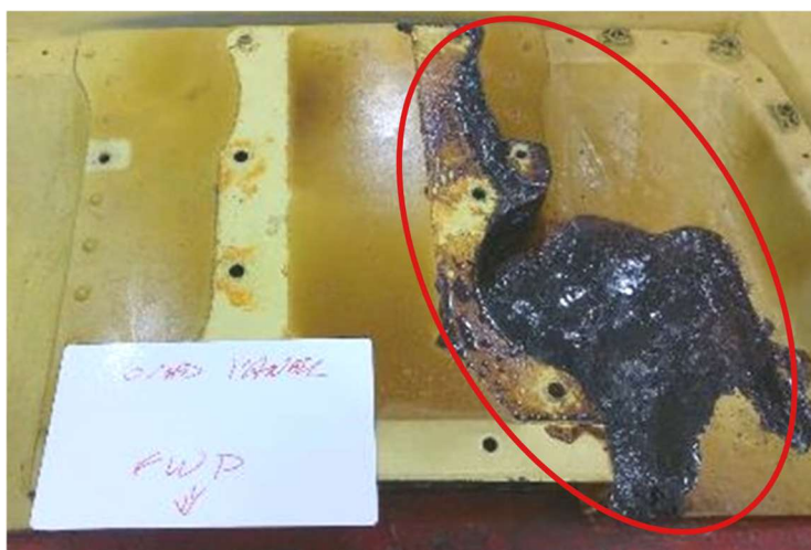
Photo 6: Melted Resin from C3 onto the Overhead Panel
