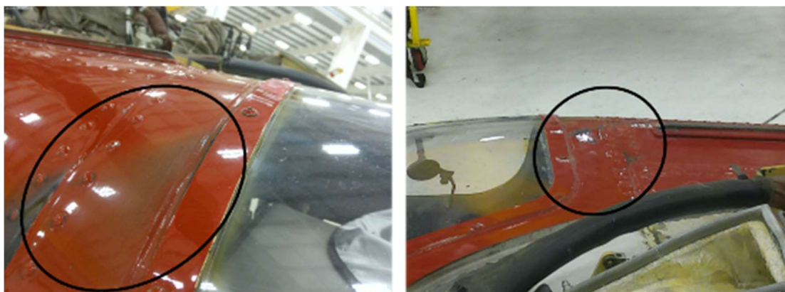
Photo 3: Soot and thermal degradation behind the greenhouse (Photo modified by NTSB).
