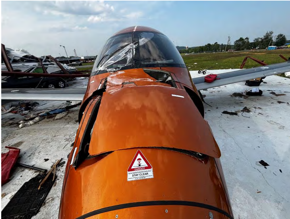
57. Component - CAPS System / Component – Moisture/Damage Beyond Repair
