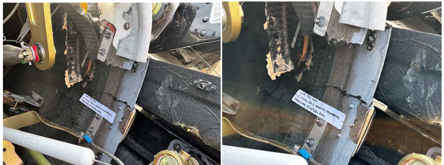
25. Fuselage - LWR Tail Skin, FS370 RBL6, Toolside / Sandwich Structure - Laminate Only - Penetrating - Fracture / 8" x 8", All Plies.
