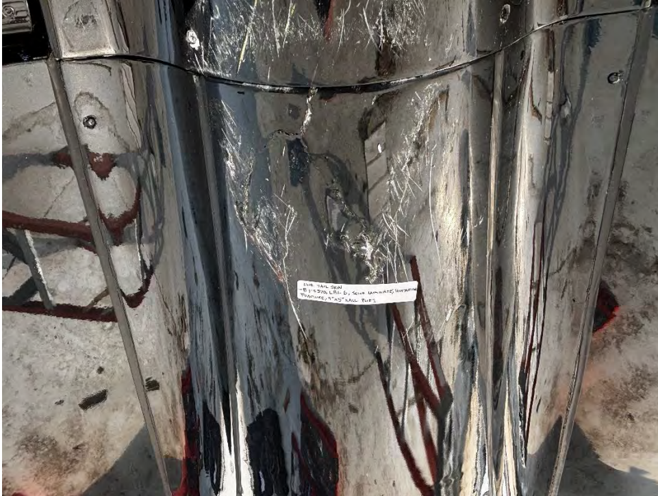
25. Fuselage - LWR Tail Skin, FS370 RBL6, Toolside / Sandwich Structure - Laminate Only - Penetrating - Fracture / 8" x 8", All Plies.
