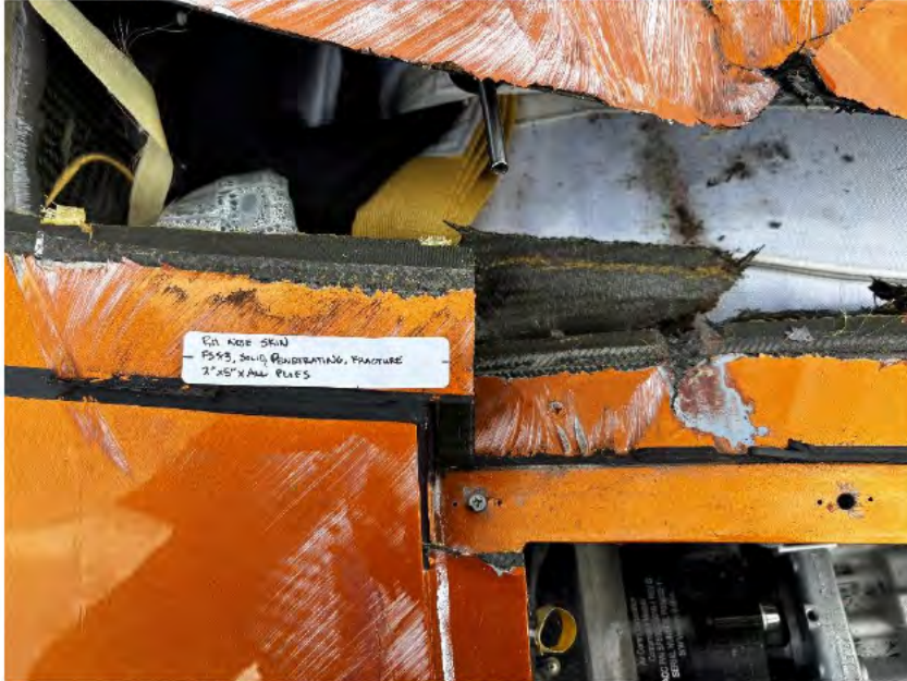
9. Fuselage - LH Nose Skin to CAPS Bucket Flange, FS78 / Secondary Bond / 2" x 2".
