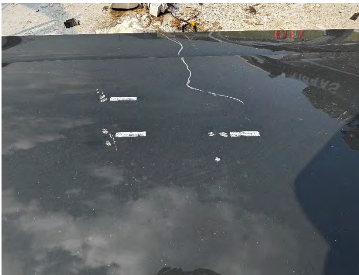
35. Wing - RH UPR Wing Skin, WS151 33" Aft of LEOP, Toolside / Sandwich Structure - Laminate Only - Penetrating - Fracture / 4" x 1", Toolside Plies Only.
