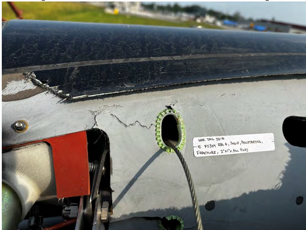
22. Fuselage - UPR Tail Skin, FS369 RBL6 / Solid Laminate - Penetrating - Fracture / 2" x 1", All Plies.
