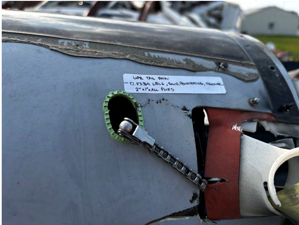
22. Fuselage - UPR Tail Skin, FS369 RBL6 / Solid Laminate - Penetrating - Fracture / 2" x 1", All Plies.
