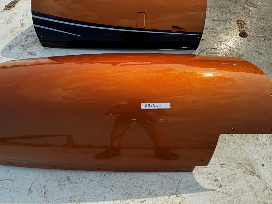
76. Composite Detail Part – LH Mid Nacelle / Component - Cosmetic / Scratches
